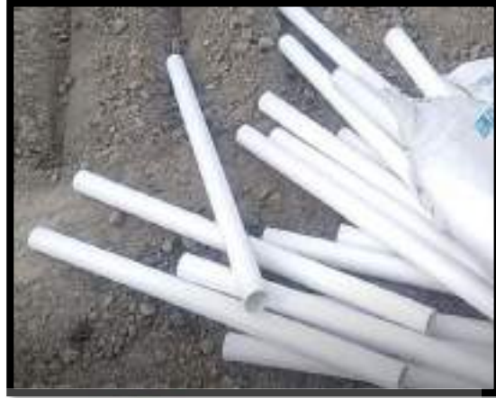
Gambar 4.3 Pipa PVC 1 Inch.
